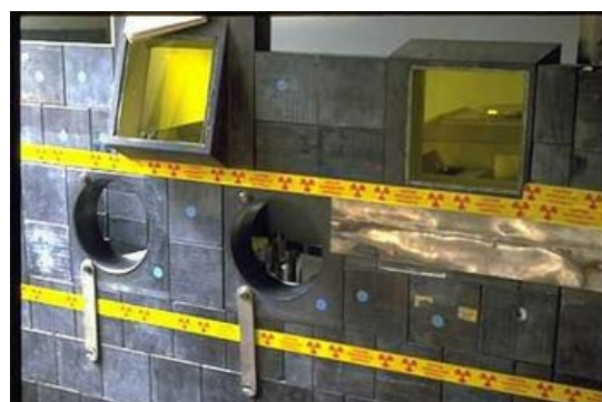
A lead cabinet where radiopharmaceuticals are prepared.
