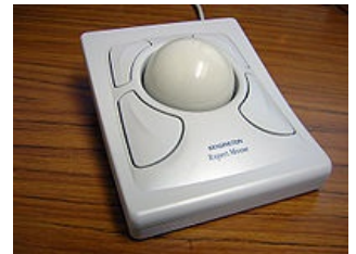
Trackball, an input device that can be easier to control than a classic mouse in some cases of movement disorders.
